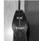
4. When the lawnmower is working ,put the Handle bar to "RUN"
