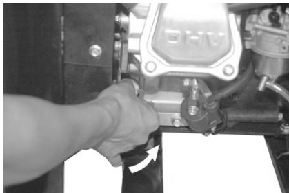
Figure 4- Unscrewing the oil cap
