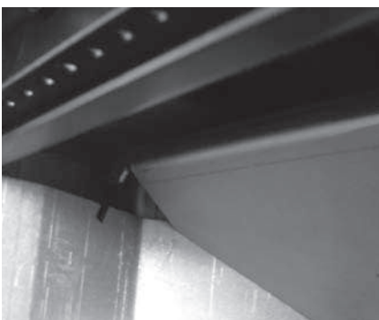
Pict. 15: Lift the fire shield
