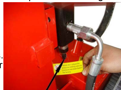
Illustration 6 Never adjust it as shown above !!
